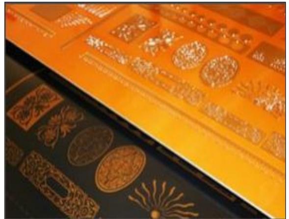
Flexographic coating plates are essential for adding protective or decorative finishes to printed materials, enhancing their appearance and durability. These finishes can provide qualities such as gloss, matte, or special effects, making them crucial in industries like label printing, packaging, and commercial printing where aesthetics and functionality are important.
