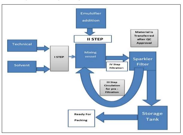
Manufacturing Process Flow Diagram For Cartap Hydrochloride 4%GR:
